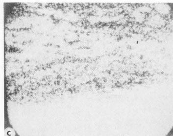
Figure 19. Electron probe analysis of corrosion product in condenser tube. (a) Secondary electron image. (b) Copper X-ray map. (c) Iron X-ray map. (Newbury and Yakowitz, 1975. Copyright, 1975 Plenum Publishing Corporation. Reproduced by permission).
