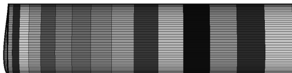
Figure 3. A view from above of a rectangular 3D wing defined with each span-wise ring of boundary faces as a separate boundary. Each shade of gray represents a different boundary patch with the endcap on the left and the root on the right.
