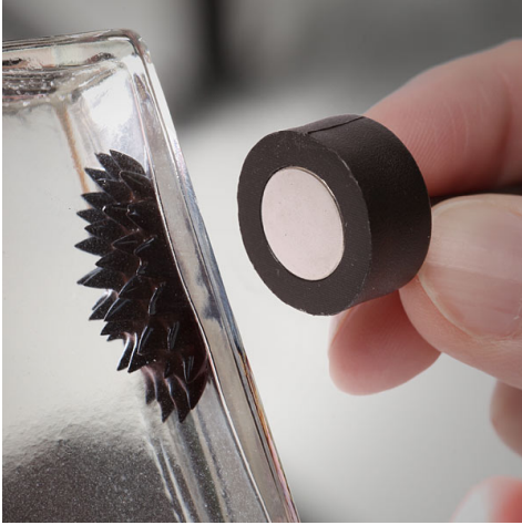
Figure 1: Ferrofluid exhibits an interesting spiking behavior when in the presence of a magnetic field.
