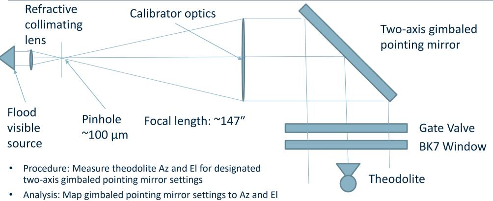
• Boresite: Set Az, El to 0,0 when the beam is normal of the UUT port flange
