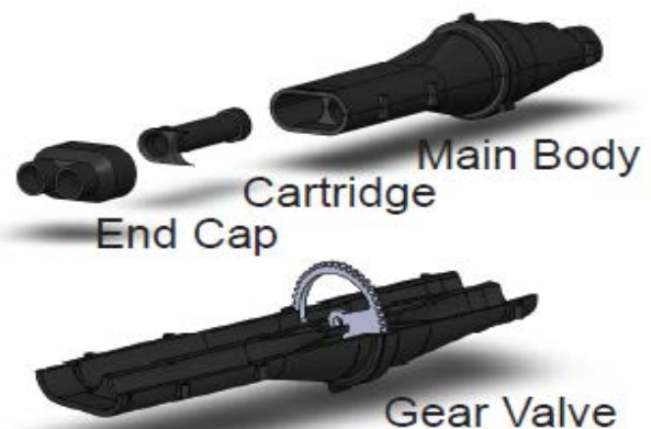
Figure 2 - 3D rendering of the prototype housing. The design includes a main body with two chambers, one of which contains a charcoal cartridge. This is contained with an end cap. Internally, a gear with a semicircle opening directs flow.
