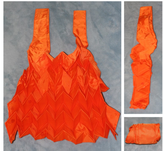
FIGURE 4: A reusable shopping bag that has been heat-set using the double mold process (including the second heat-set step) that can be easily rolled up after collapsing the origami pattern for simple storage.
