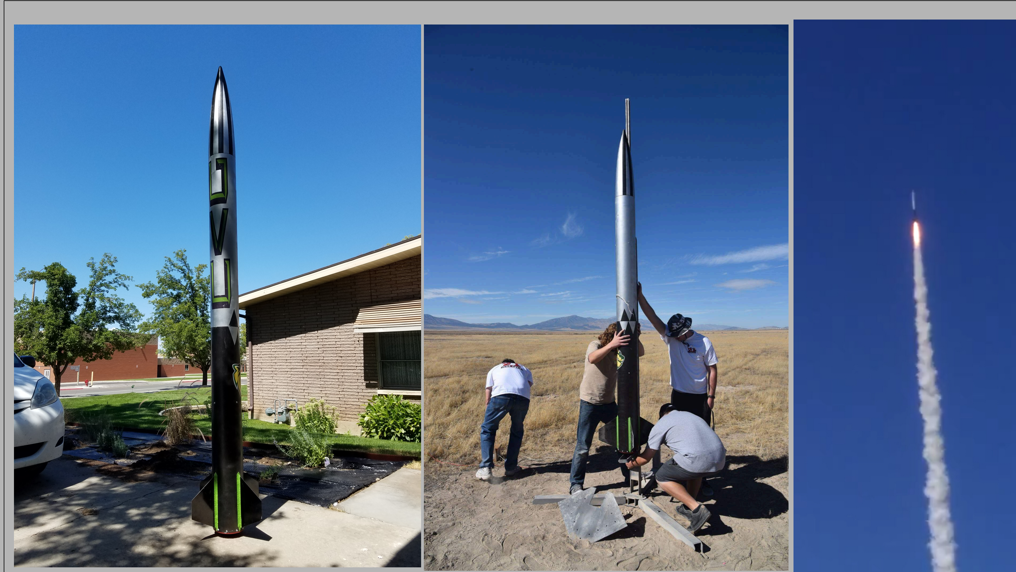
With the gained experience, a large level 3 rocket was attempted. Designed from scratch, Eric Davis successfully flew a Tripoli L3 certification flight. Tripoli is the sanctioned organization for high-powered amateur rocketry and L3 is the highest level achievable. This particular rocket reached 8,000 ft.
