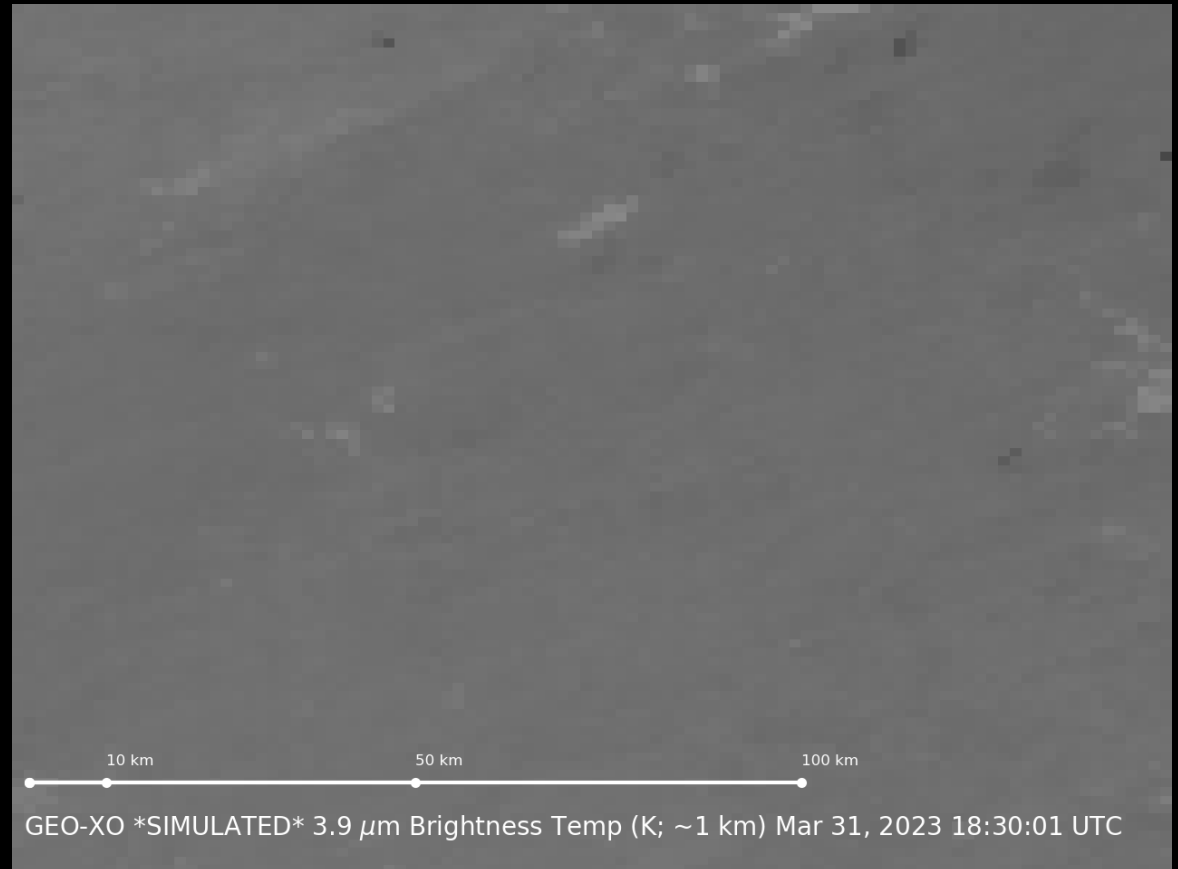
Simulated 3.9 \mu\text{m} 1 km resolution band from GXI for the same times as the ABI loop. It's based on 4 VIIRS passes from 1830, 1921, 1943, and 2012 UTC
