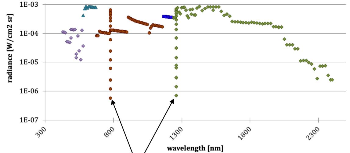
Linearity measurements at 780nm and 1260nm to characterize Si and PbS detectors
