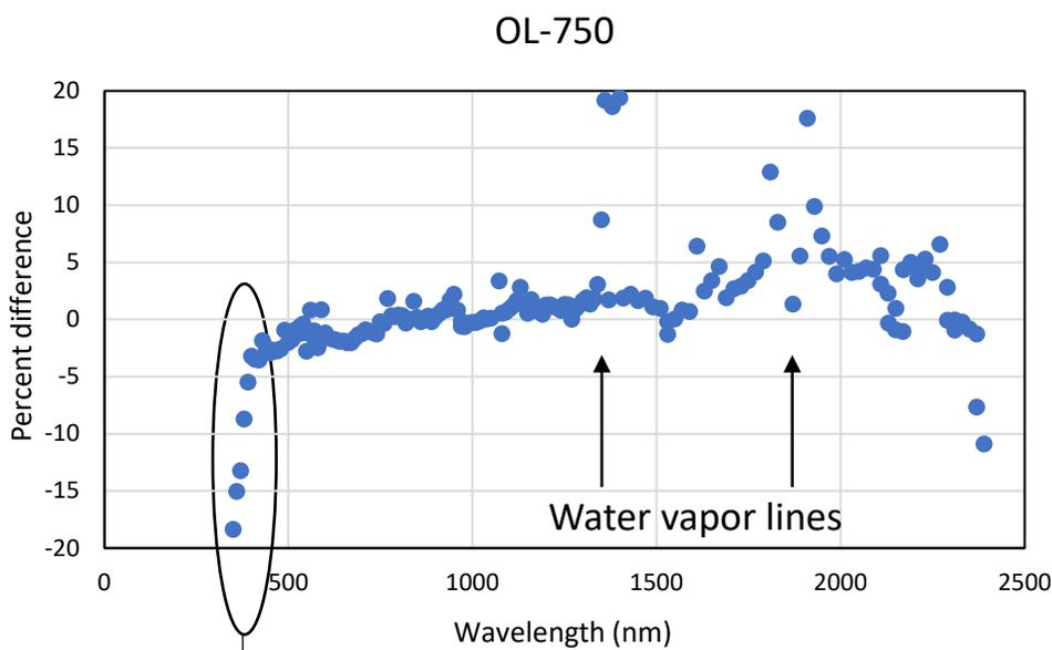
OL-750 calibration comparison between FEL lamp and GLAMR sphere
