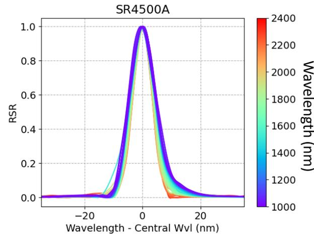
OL-750 has triangular line shape: width varies with grating configuration
