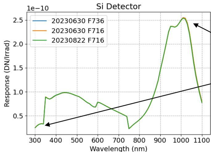
Large drop in responsivity in UV range compounds stray light contribution: OL-750 most sensitive where lamp is brightest, least sensitive where lamp is dimmest
