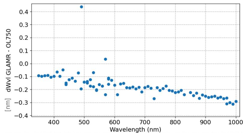
Slight drift in wavelength calibration
