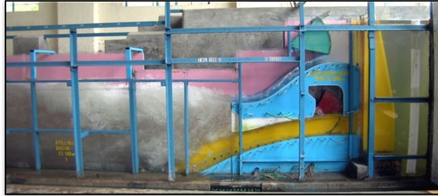
Figure 2. View of the sectional model of two tier spillway
