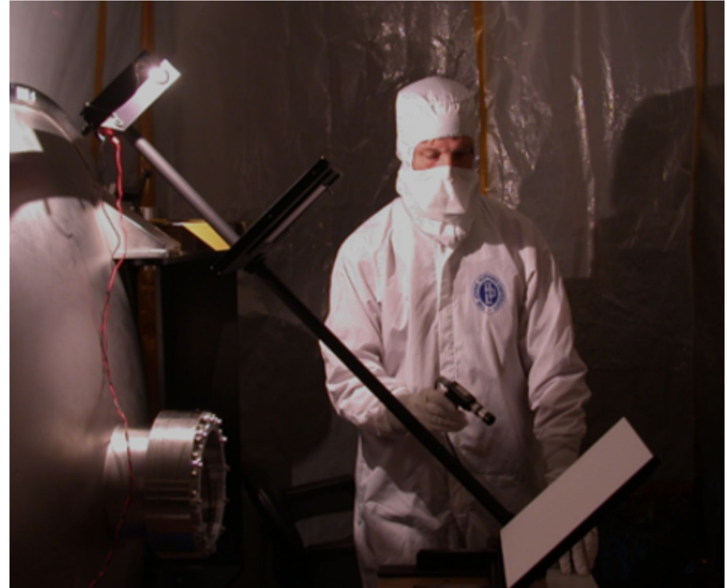
Example lab setup in which a QTH lamp illuminates a Spectralon Panel in front of the TVAC window. (Image Credit: R. Green, JPL)
