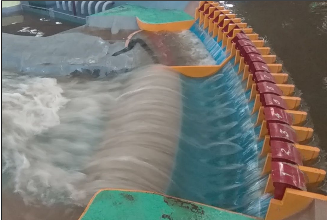
Photo 6. Performance of ski jump bucket, Q= 32872 \text{ m}^3/\text{s} at Full Reservoir Level (FRL) El. 262.13 m
