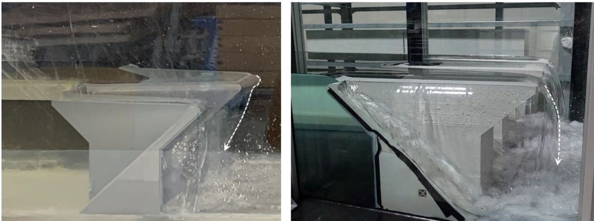
Figure 6. Scale effects and its influence on nape trajectory for comparable discharges ( H_t P^{-1} = 0.05 ), left: P 20 model, right: P 40 model
