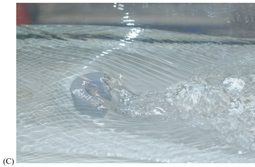
Figure 4. Flow patterns around a fully-submerged horseshoe element for d_1/H \sim 1.4 . (A) Model L4, d_1/H = 1.445 , Q = 0.0447 \text{ m}^3/\text{s} ; (B) Model M4, d_1/H = 1.38 , Q = 0.0121 \text{ m}^3/\text{s} ; (C) Model M1, d_1/H = 1.4 , Q = 0.0128 \text{ m}^3/\text{s} .
