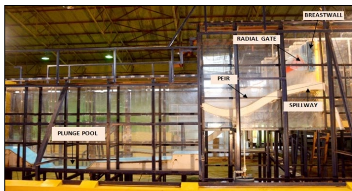
Figure 1 (a). Side view of the dry physical model (1:50 scale) of spillway and plunge pool for original design of spillway.
