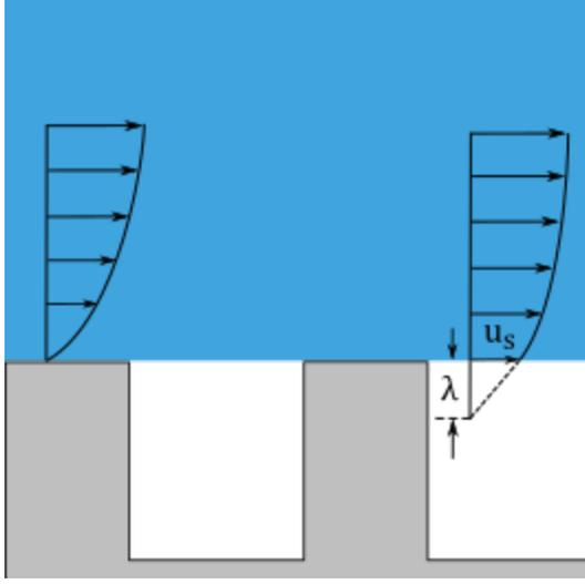
**FIGURE 3.** Demonstration of Different Boundary Conditions on SH surfaces.
