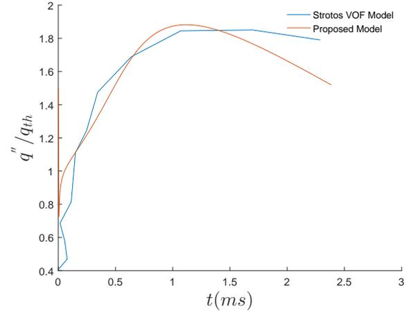
**FIGURE 6.** Heat Flux normalized by 1D Conduction Solution for Clavijo et al. model and Strotos VOF model for reference case.
