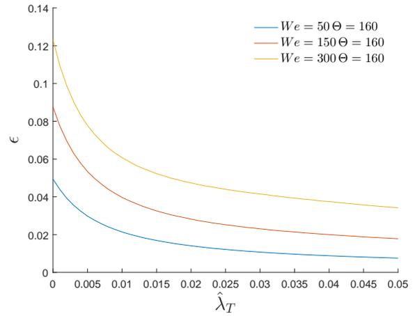
**FIGURE 9.** Cooling Effectiveness for Clavijo et al. model and Strotos VOF model for reference case.
