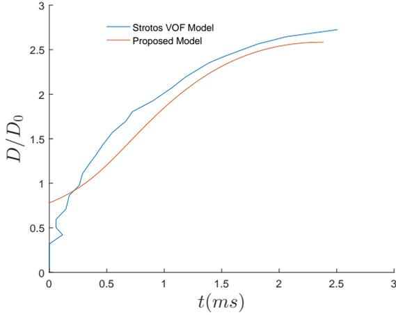
**FIGURE 5.** Diameter vs Time during expansion for Clavijo et al. model and Strotos VOF model for reference case.
