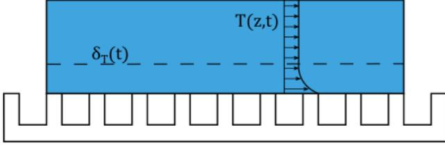
**FIGURE 4.** Control volume visualization for impingement model for SH surface using integral method. The energy is stored in the drop by allowing the boundary layer thickness,  $\delta_T$ , to change with time.
