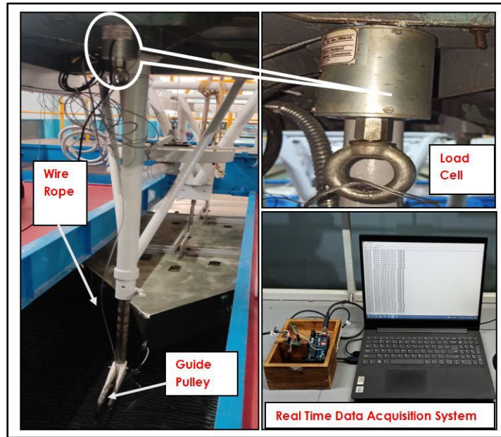
Figure 4. Experimental setup along with load cell and data acquisition system
