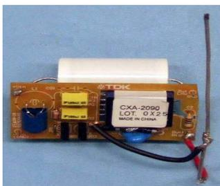
Fig 8- The Micro-Pulsed Plasma Thruster
