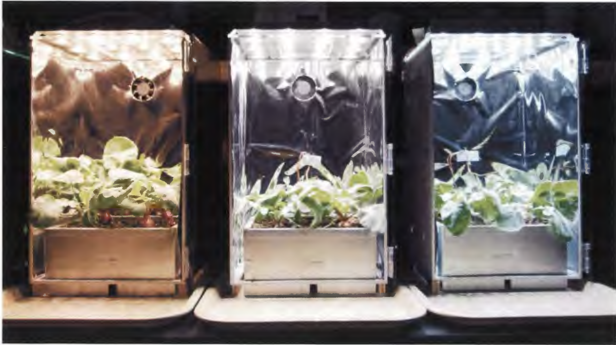
Figure 1. Experimental set-up showing growth chambers, LED arrays, root modules, and thermocouples. The crop shown is radish on the day of harvest. Note the differences in plant form across treatments, which are arranged (left to right) warm, neutral, and cool white LEDs.
