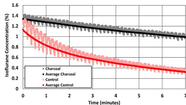
**Figure 5** - The observed concentration of isoflurane during ventilation between 10 grams of activated charcoal and the test lung. Activated charcoal (grey) allowed for the gradual release of isoflurane compared to the control (pink). A running average is shown for both the activated charcoal (black) and control (red).
