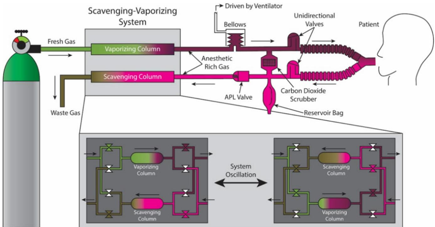
**Figure 6** - Schematic of the proposed Scavenging-Vaporizing System and how it functions with a commercial ventilator. Within the system exists two columns alternating in function between vaporizer and scavenger. These roles are determined through the actuation of valves. Not shown is an anesthetic gas reservoir used if neither column can deliver the set concentration of anesthetic, as well as a fresh gas bypass for when no anesthetic is needed.
