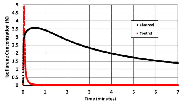
**Figure 4** The observed concentration of isoflurane leaving the vessel containing 40 grams of saturated activated charcoal as the flow was reversed at 2 liters per minute. The activated charcoal (black) allowed for the gradual release of isoflurane compared to the control (red) containing no activated charcoal.
