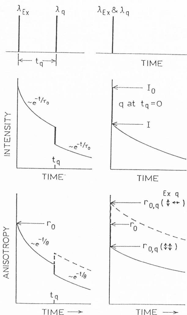
**Figure 15.** Schematic of light quenching by a time-delayed quenching pulse. The dotted lines refer to light quenching with perpendicular polarized light.
