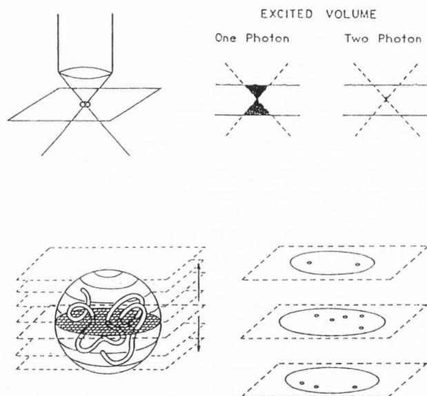
**Figure 11.** Intrinsic "confocal" excitation using TPIF in microscopy (top) and three-dimensional optical imaging (bottom).
