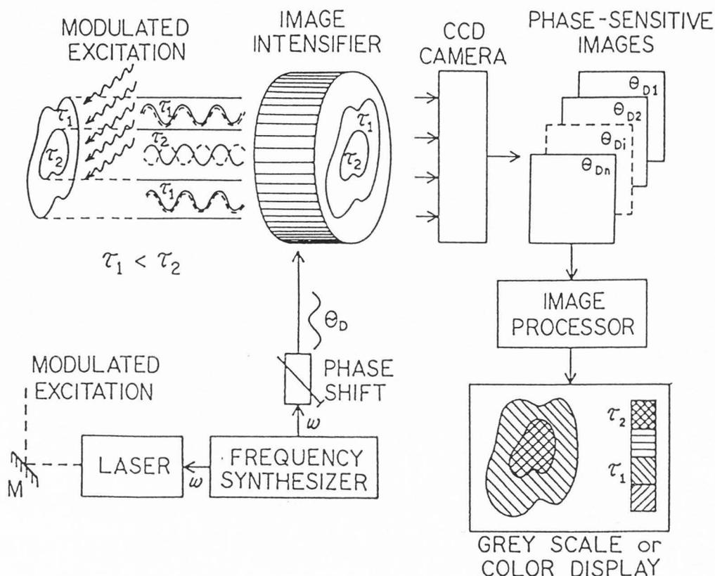
Figure 3. Apparatus for fluorescence lifetime imaging microscopy (FLIM).
