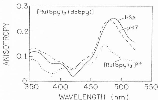
**Figure 6.** Excitation anisotropy spectra (bottom) of  $[\text{Ru}(\text{bpy})_2(\text{dcbpy})]$ , free (---) and when conjugated to HSA (—). The anisotropy spectra are in glycerol:buffer (9:1, v/v) at  $-55^\circ\text{C}$ . This viscous solvent is used to prevent rotational diffusion during the excited state lifetime. The dotted lines (.....) represent the symmetrical  $[\text{Ru}(\text{bpy})_3]\text{Cl}_2$ .
