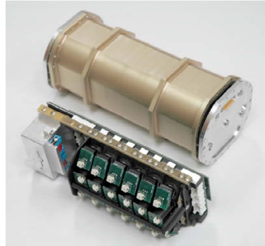
Figure 3 GeneSat-1 payload pressurized volume showing optical bench
