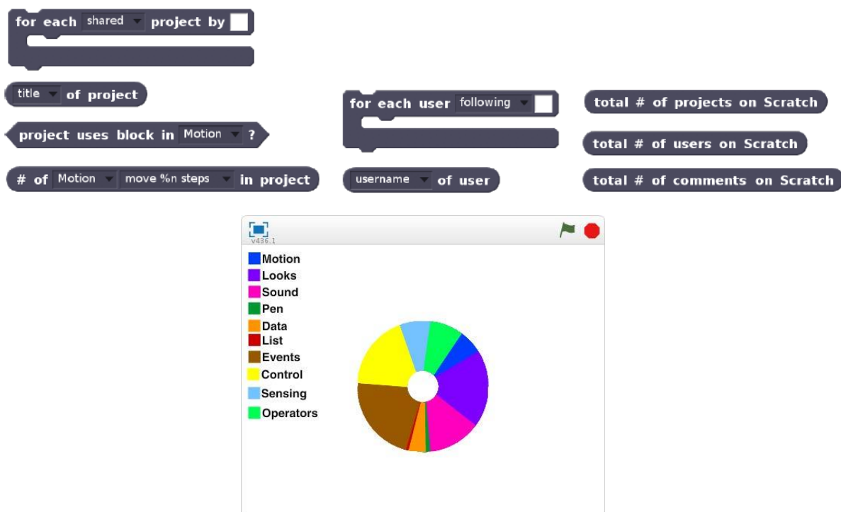
Figure 2. The set of data blocks that enable data queries from Scratch users (above) and a resulting Scratch data visualization showing total distribution of different block-type usage by the Scratch community, provided by Sayamindu Dasgupta.
