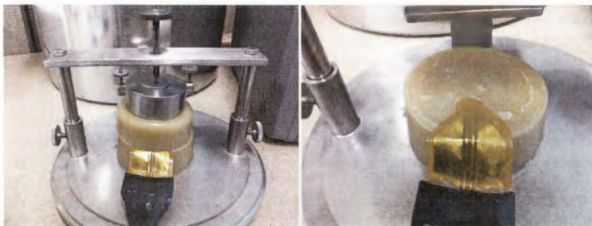
Figure 4: HotDisk© Experimental Set-up for Measuring Solid Thermal Properties
