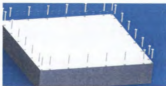
Figure 2: Bolting Top Plate to Aluminum Box
