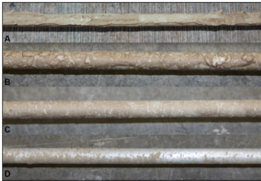
Figure 6. Airepel® HC with castor oil-treated aluminum perches used for repellent efficacy testing with European starlings ( Sturnus vulgaris ) at the National Wildlife Research Center's Outdoor Animal Research Facility, Fort Collins, Colorado, USA, 2016–2018. (A) Airepel HC with castor oil formulation before exposure to birds; (B) Airepel HC with castor oil formulation after exposure to birds showing minimal wear; (C) Airepel HC with castor oil formulation after exposure to birds showing moderate wear; (D) Airepel HC with castor oil formulation after exposure to birds showing heavy wear (photos courtesy of H. McLean).
