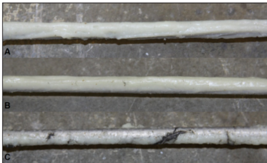
Figure 7. MS2-treated aluminum perches used for repellent efficacy testing with European starlings ( Sturnus vulgaris ) at the National Wildlife Research Center's Outdoor Animal Research Facility, Fort Collins, Colorado, USA, 2016–2018. (A) MS2 formulation before exposure to birds; (B) MS2 formulation after exposure to birds showing minimal wear; (C) MS2 formulation after exposure to birds showing moderate wear (photos courtesy of H. McLean).
