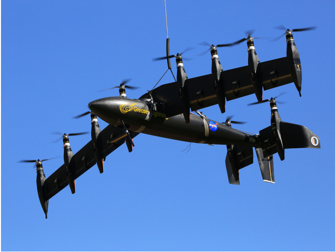
FIGURE 1: The NASA Greased Lightning (GL-10) prototype in hover mode. Credits: NASA Langley, Dave Bowman.
