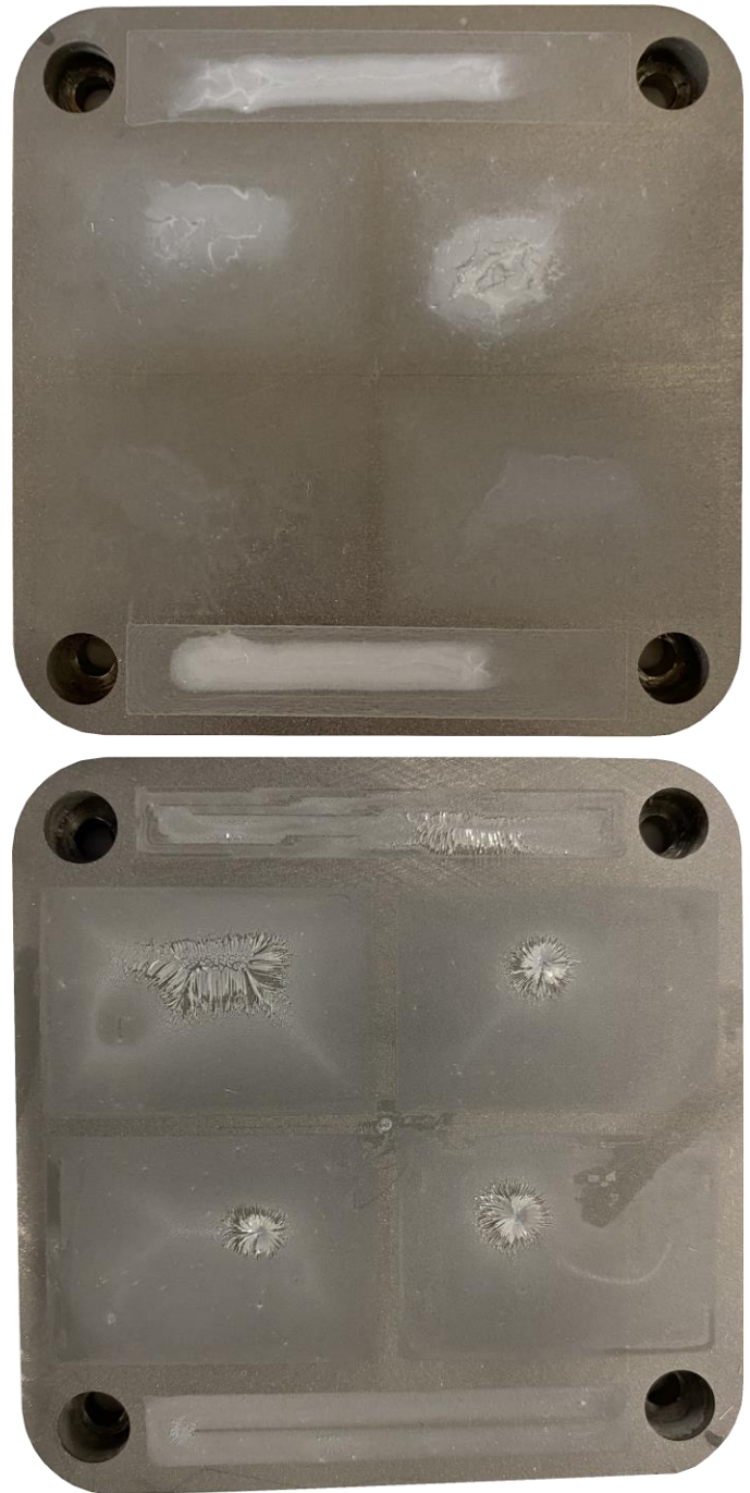
Figure 9 - Dried alumina (top) and zirconia (bottom) deposits performed using direct write deposition.
