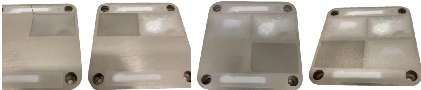
Figure 8 - Recently deposited liquid alumina slurry in different concentrations. Left to right: 3 wt%, 2 wt%, 1 wt%, and 0.5 wt% slurry.
