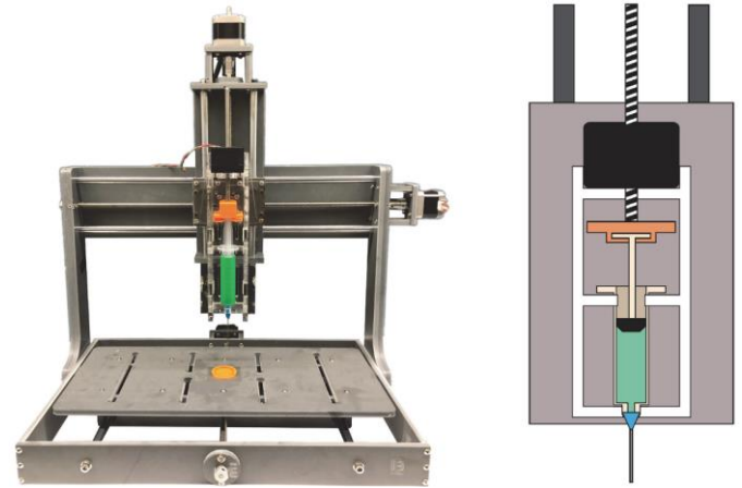
Figure 3 - Direct write deposition system (image from Romero et al. [1] used with permission). The three-axis stage controls the deposition location while the stepper motor above the syringe controls the rate of material ejection from the needle onto the substrate.
