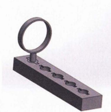
Figure 12. First design of the ultrasound holder. This holder consists of multiple locking notches and required the holder to have a matching piece to ensure proper locking.
