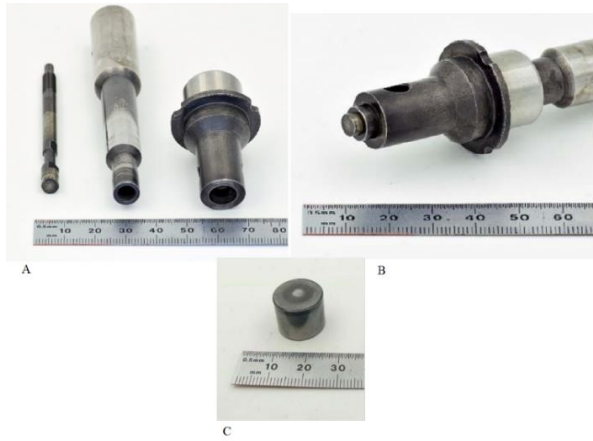
Fig. 4: RFSSW tools and anvil.
