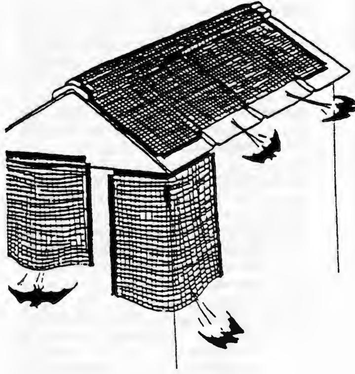
Figure 1. Plastic industrial birdnetting ( $\frac{1}{2} \times \frac{1}{2}$  inch mesh size) used to exclude bats from buildings (a) can be used in many situations (b).
