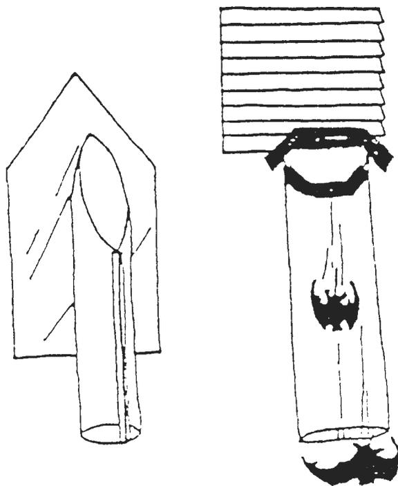
Figure 4. Collapsible sleeves made from a sheet of heavy plastic can be used to exclude colonies that use small roost exits. This inexpensive excluder works best when there is little or no wind. To prevent suffocation of bats in tight roosts, this device should be installed just before dusk.
