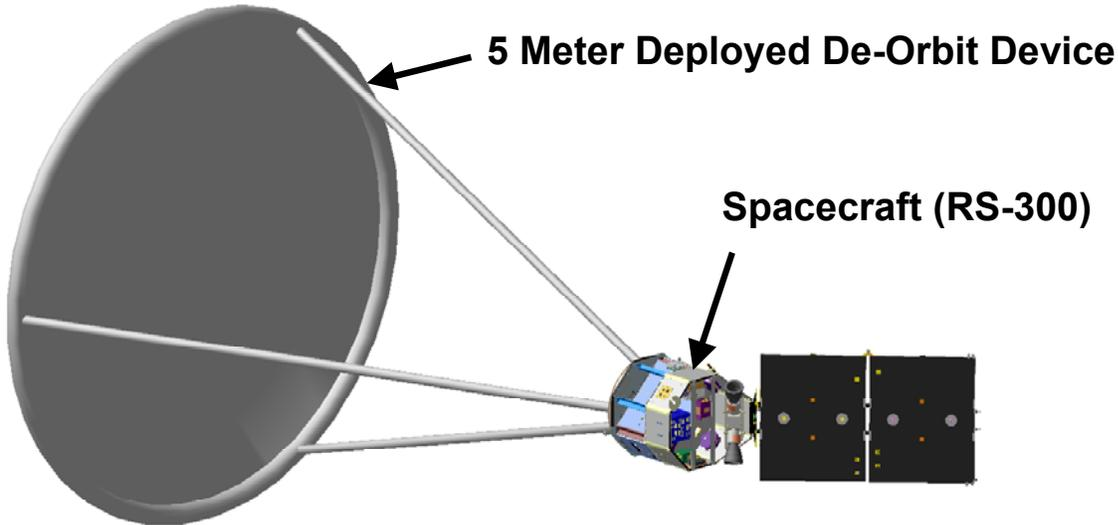
**Figure 2.4-1 Payload Configuration (5 m Deployed)**
