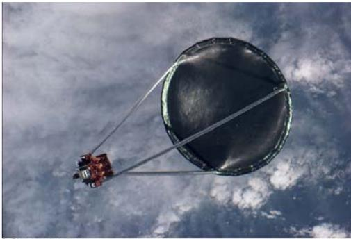
**Figure 2.2-2. L'Garde Inflatable Antenna**
