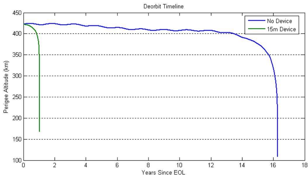
**Figure 2.5-5 Orbital Decay of SV Using a Aerobraking Maneuver (15 m De-orbit System)**
