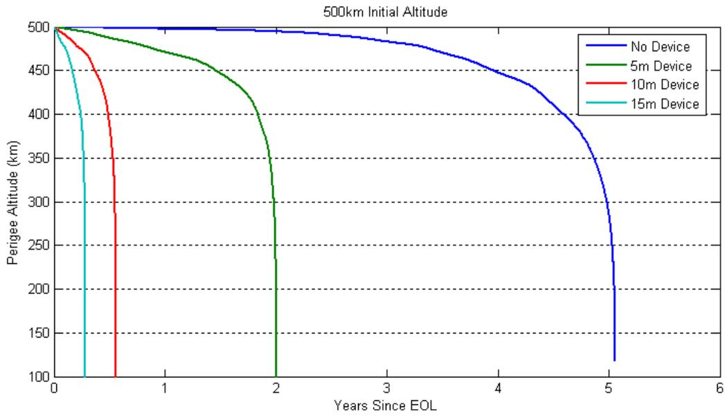
Figure 2.5-2 Orbital Decay of SV w/wo De-Orbit Payload (500 km circular altitude)
