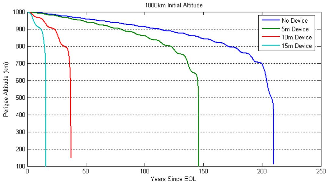
**Figure 2.5-4 Orbital Decay of SV w/wo De-Orbit Payload (1000 km circular altitude)**
