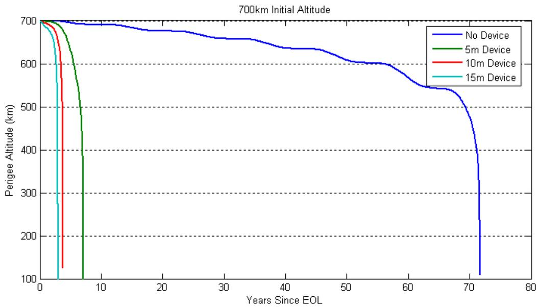
Figure 2.5-3 Orbital Decay of SV w/wo De-Orbit Payload (700 km circular altitude)
