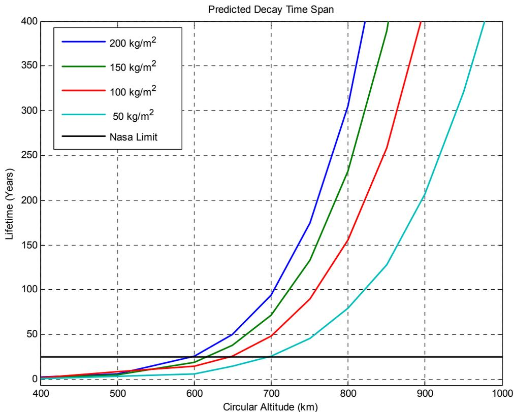
**Figure 2.5-1 Orbital Decay vs. Altitude with respect to  $B^*$  (kg/m<sup>2</sup>)<sup>a</sup>**
