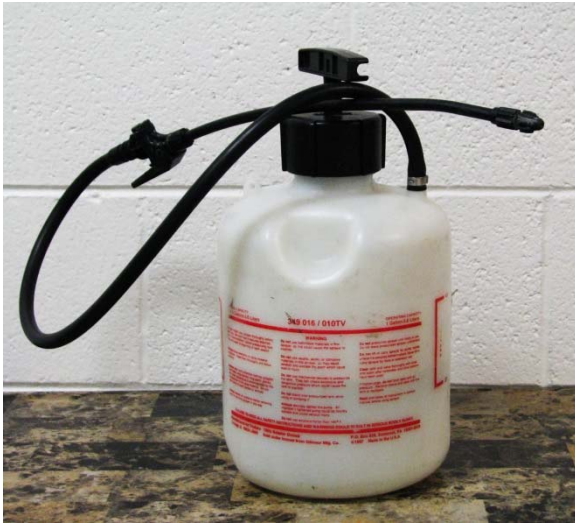
Figure 4. Small hand sprayer that can be used to spray disinfectant solution on small objects.
