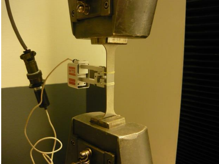
Figure 1. Tensile testing setup for DMLS parts
