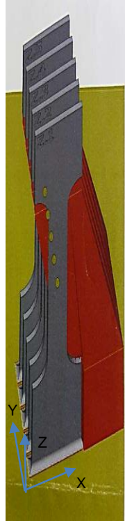
Figure 3. DMLS tensile specimens printed in the vertical direction (Z-direction). Red represents support structure required.
