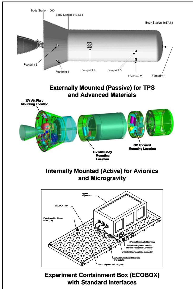
**Figure 3. K-1 Technology Experiment Accommodations**
