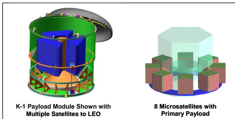
**Figure 2. Multiple Small Satellites on the K-1**
