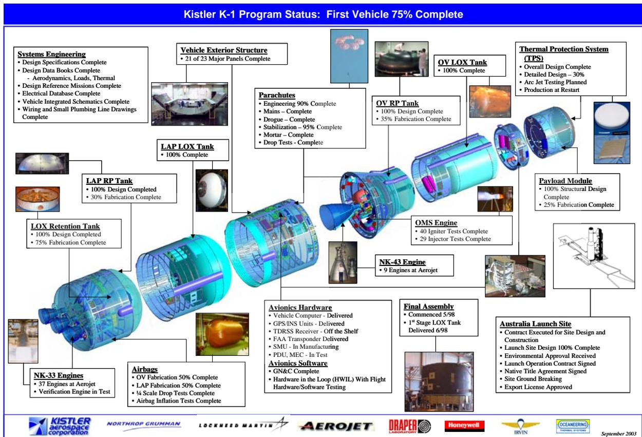
**Figure 6. K-1 Hardware is 75% Complete**
