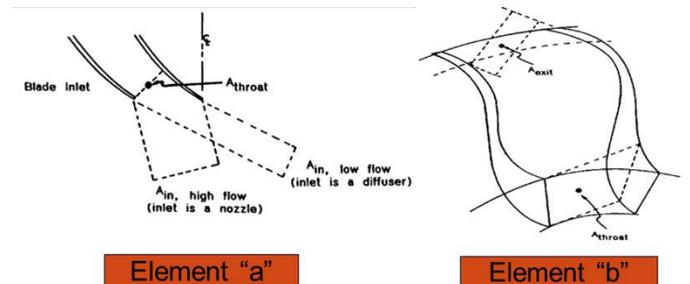
**FIGURE 2:** A VISUAL DESCRIPTION OF THE TEIS MODEL, SHOWING THE INLET (ELEMENT A) AND THE BLADE PASSAGE (ELEMENT B) [1].
