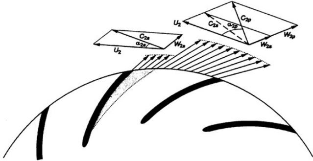
**FIGURE 1:** A CONCEPTUAL REPRESENTATION OF THE TWO-ZONE MODEL, SHOWING PRIMARY AND SECONDARY VELOCITIES. NO IMPLICATION OF THE PHYSICAL LOCATION OF THE TWO ZONES IS INTENDED BY THIS SKETCH [1].
