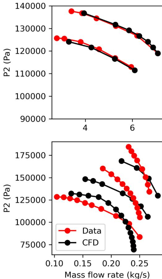
**FIGURE 5:** THE IMPELLER OUTLET PRESSURE AS A FUNCTION OF MASS FLOW RATE. VALUES SHOWN ARE FROM EXPERIMENTS AND CFD FOR A LOW-SPEED (TOP) AND HIGH-SPEED (BOTTOM) IMPELLER.
