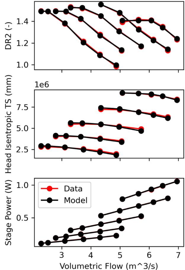
**FIGURE 3:** A COMPARISON OF THE DIFFUSION RATIO, THE HEAD RISE, AND THE STAGE POWER CALCULATED BY THE MODEL TO THE MEASURED VALUES.
