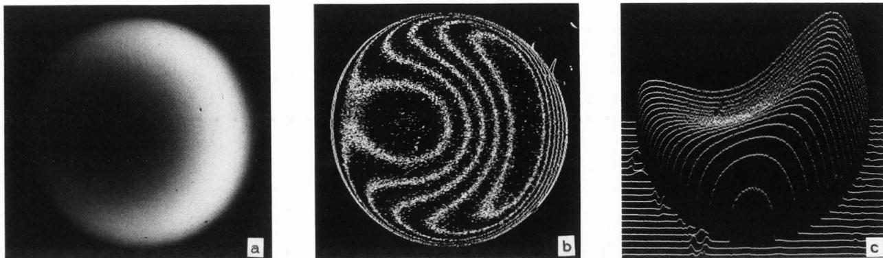
Fig. 4 Images of a 0.9 mm steel ball taken with a ring detector for BSEs. (a) - normal image, (b) - isodensities, (c) - Y-modulation image of a lower half of the ball.  $U_0=20$  kV,  $WD=15$  mm.
