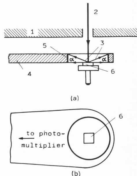
**Fig. 1** Schematic diagram of the ring detector (a) - cross section, (b) - top view. 1- microscope lens, 2- primary beam, 3- backscattered electrons, 4- light guide, 5- layer of scintillator, 6- specimen.  $\alpha$  is an acceptance angle of the detector.
