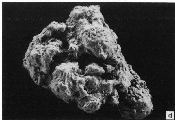
Fig. 3 A comparison of images taken with the ring detector for BSEs and the E.T. detector for SEs. (a) and (c) - SE images, (b) and (d) - BSE images, (a) and (b) - a surface of chemically etched GaAs wafer, (c) and (d) - an iron grain.  $U_0 = 20$  kV,  $I_0 = 4 \cdot 10^{-10}$  A, untilted specimens, WD = 17 mm.
