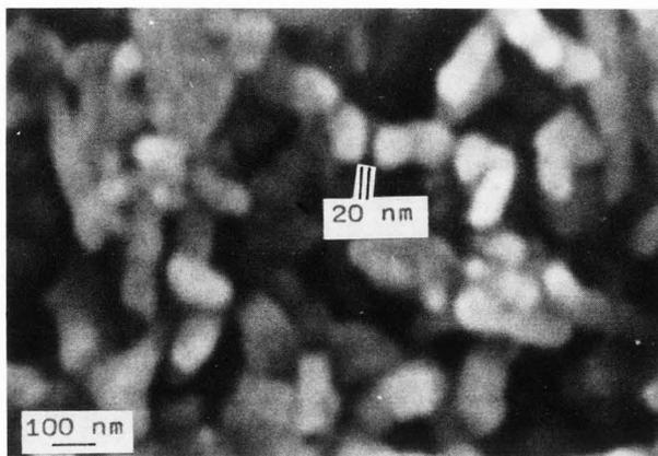
Fig. 2 An image of a gold coated magnetic tape taken with the ring detector.  $U_0 = 40$  kV,  $I_0 = 5 \cdot 10^{-10}$  A, untilted specimen, WD = 15 mm.
