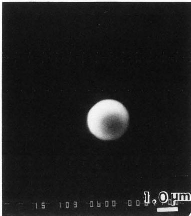
Fig. 4. Alloy spherical particle micrography. Diameter, 1.8  $\mu\text{m}$ ; substrate, polished graphite piece.
