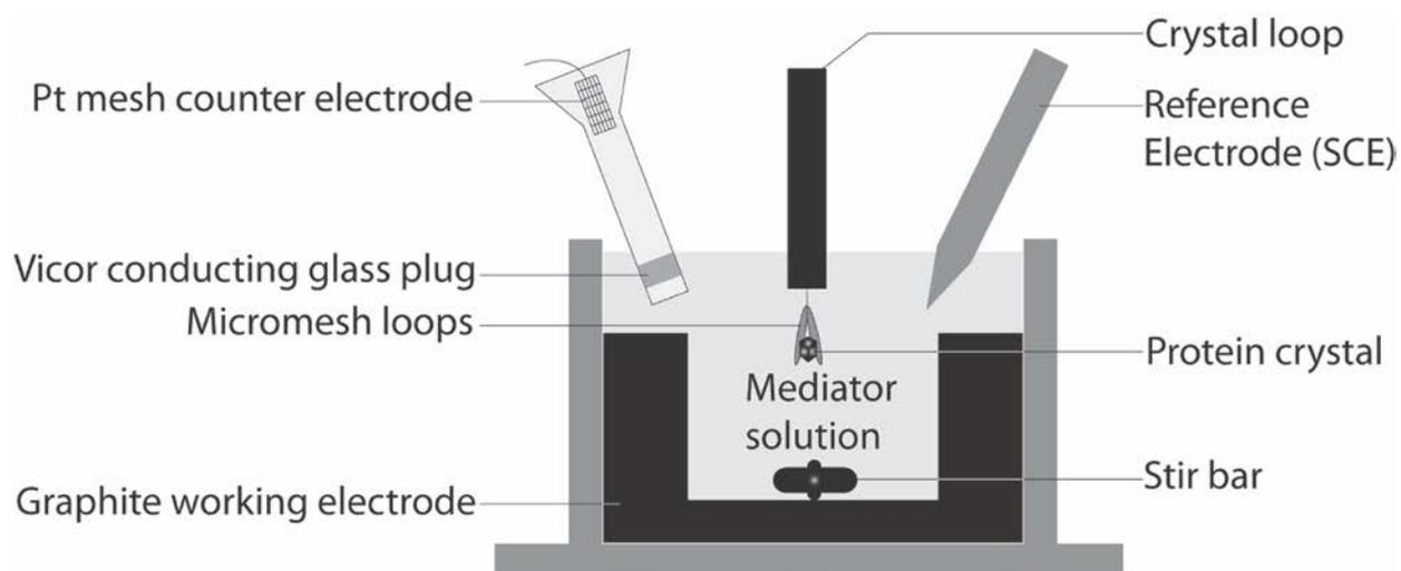
**Figure 2.** Schematic diagram of the crystal potential poising apparatus. Crystals were submerged in a stirred solution held at constant potential for 1 hour prior to flash cooling in liquid nitrogen to poise them in distinct structural states.
