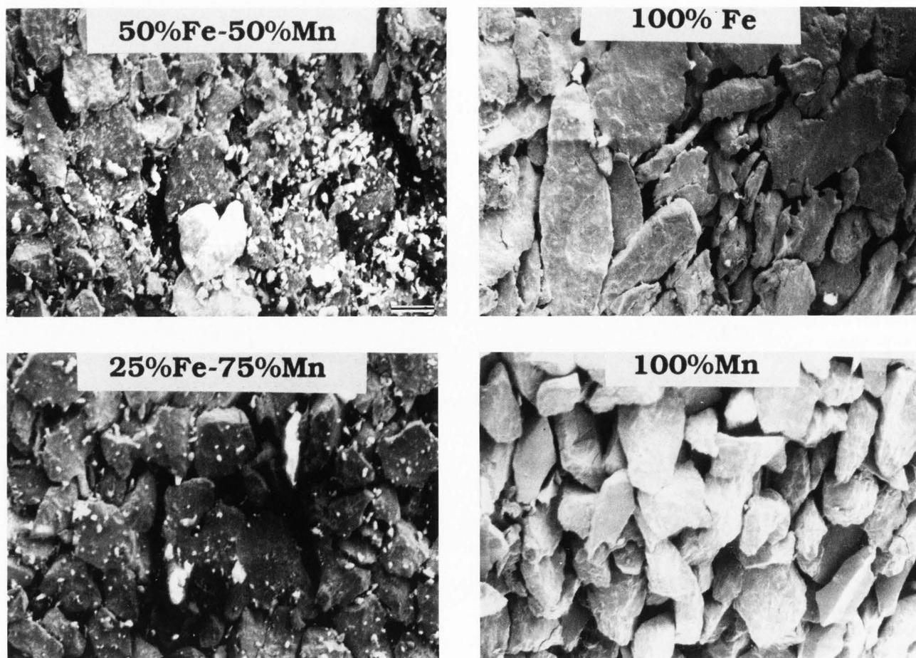
**Figure 2 (above).** Scanning electron micrographs show that the surface of the bulk of 50% Fe-50% Mn mixture has features of both pure iron, and pure manganese. Bars = 100  $\mu$ m.
