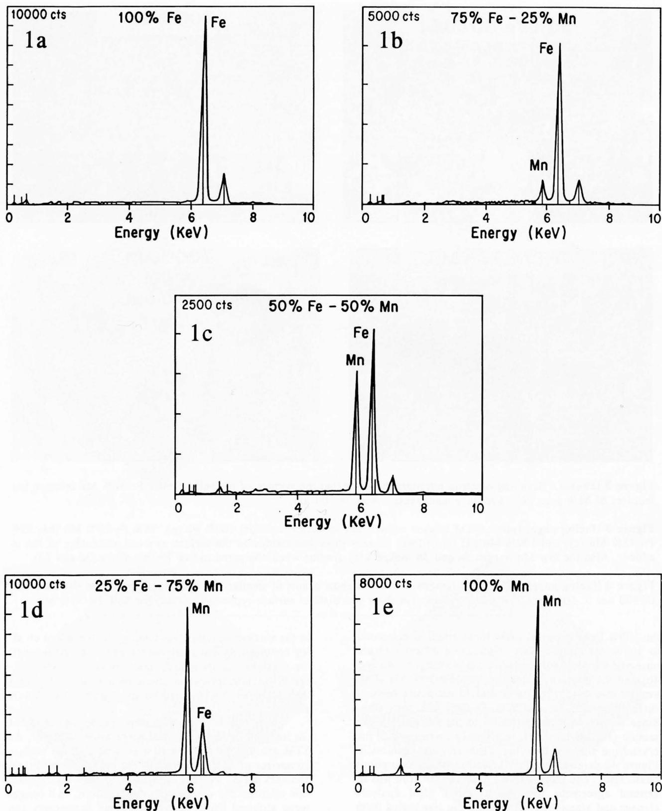
Figure 1: The composition of the bulk alloy prepared by electro-discharge compaction for various composition is shown: a: 100% Fe; b: 75% Fe-25% Mn; c: 50% Fe-50% Mn; d: 25% Fe-75% Mn; and e: 100% Mn.
