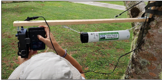
Figure 4. Bait tube and bracket emulating a tree branch with a time lapse trail camera set to monitor baits. Monitoring of brown treesnake ( Boiga irregularis ) baits occurred on Andersen Air Force Base, Guam, from May 18 to October 6, 2020.
