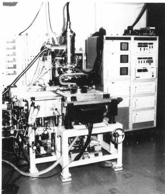
**Figure 2.** A photograph of the prototyped electron beam lithography system.
