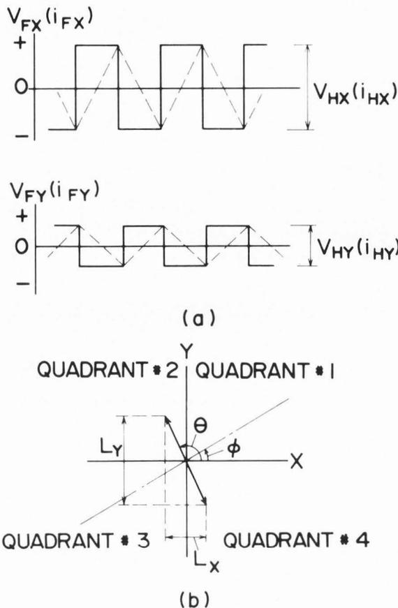
Figure 8. The signals which are out of phase 180 degrees (a; top) and a movement of electron beam (b; bottom).
