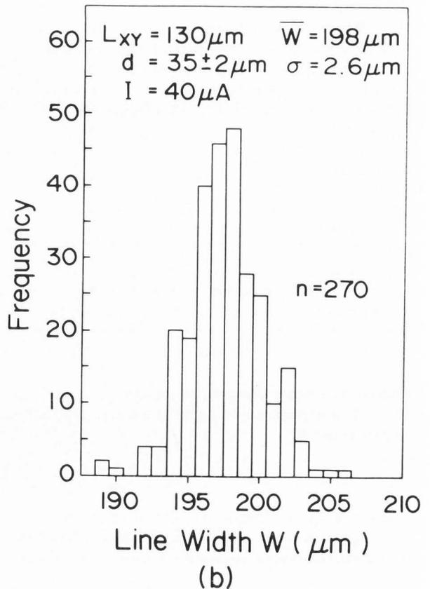
was 2  $\mu\text{m}$ . These data led to the conclusion that the present control system is able to write the lines of various widths with considerable accuracy, well suited for the fabrication to printed wiring boards.
