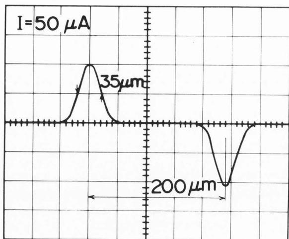
**Figure 1.** A measured beam profile at a beam current of  $50 \mu\text{A}$ .
