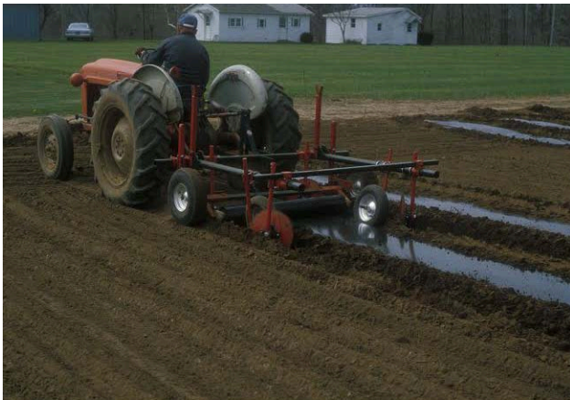
Figure 1. Single-row plastic layer pulled by tractor.
