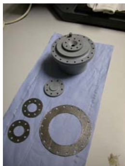
Figure 8. Solar receiver and graphite foil (Grafoil) gaskets.
