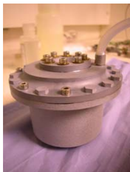
Figure 9. Sealed solar receiver undergoing 3.9 bar leak check.
