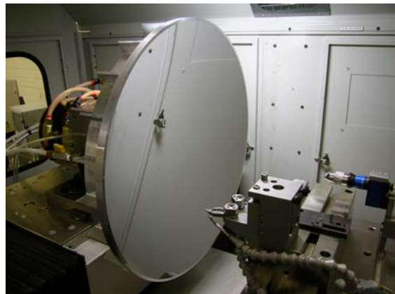
Figure 14. 56-cm aluminium concentrating mirror on diamond turning tool following fabrication.
