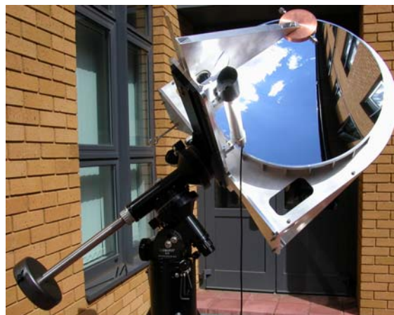
Figure 17. Optical test rig mounted on Losmandy GM-11 mount.
