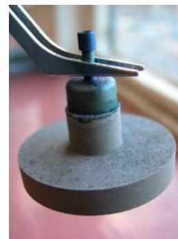
Figure 13. Braze test specimen, Mo/Ru filler, Mo cap, IMC post. Pressure = 1-2 mbar.
