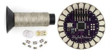
*Note:* (left) LilyPad basic e-sewing kit: Conductive thread, battery holder, 3V coin cell battery, push button switch, light emitting diode (LED); (right) LilyPad Arduino microcontroller
