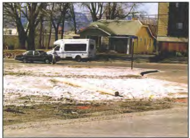
A thin snow-like layer of salt will often rise to the surface of Mancos Shale soils in times of extreme dryness.
