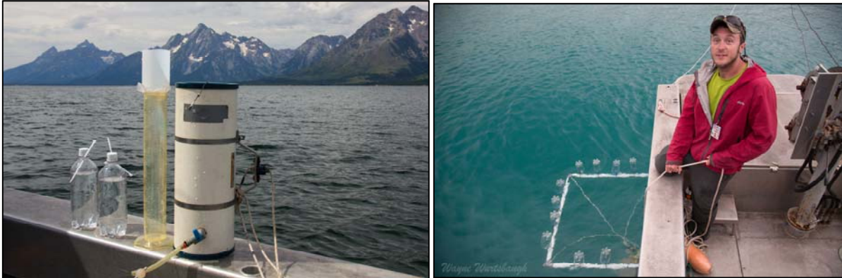
Figure 2. Left—apparatus used to collect bioassay water (Jackson Lake photo from 2014). Right—incubation frame used to incubate the 15 bioassay bottles.
