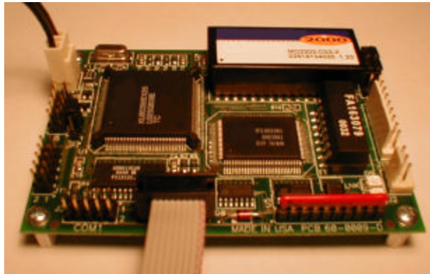
Figure 19 Picture of Skippy, the satellite computer on a board.
