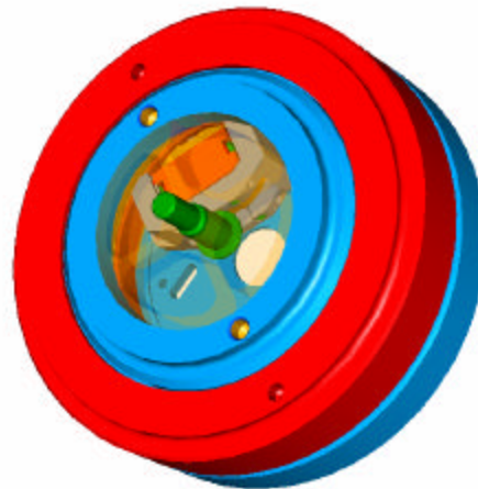
Figure 7: Rotary motor configuration with internal Ultrasonic Piezo Drive unit (top cover not shown)
