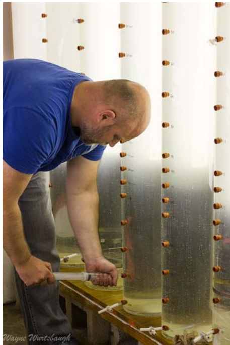
Fig. 1 Sampling deep brine layer water through a port near the bottom of the experimental columns. For this photo and for sampling, we removed the black plastic covering the bottom 50 cm of the columns
