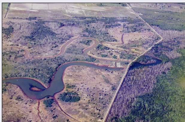
Figure 3. Trinity Inlet, Cairns, Queensland, Australia. The levee wall used to impound the wetlands is on the right. Degradation of vegetation is evident on both sides of the levee wall. Acid was released, soil C org was remineralized, and there was a 1.3 m loss in soil elevation (Hicks et al. 2003).
